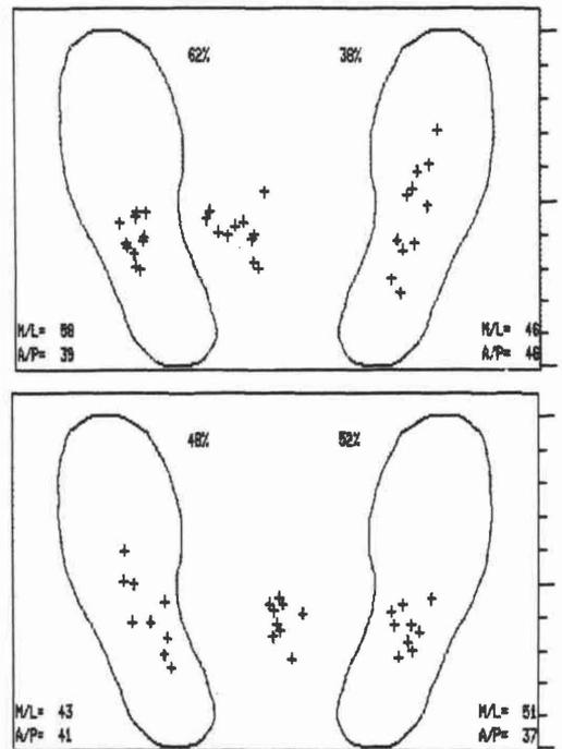
Fig. 6. Top, scattergram from 11 right above-knee amputees, wearing a variety of different limbs. Bottom, scattergram from 9 left below-knee amputees, wearing PTB prostheses with polypropylene sockets.
