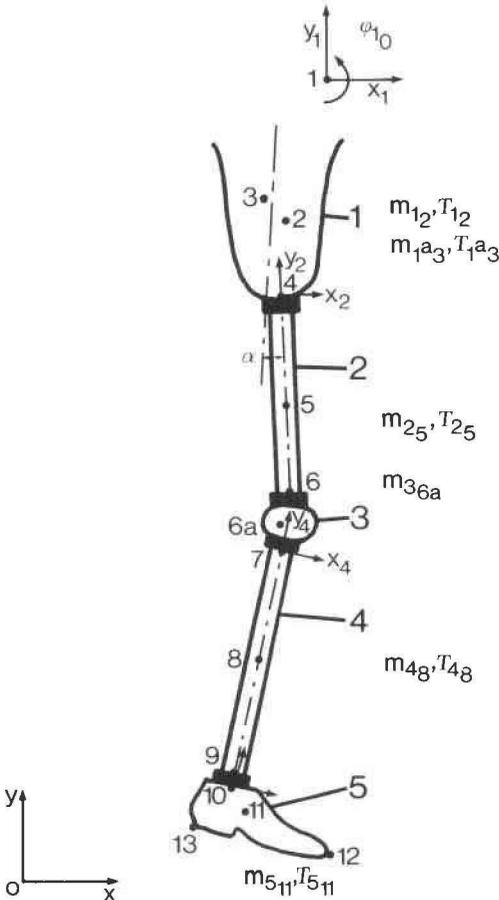
Fig. 1. The prosthesis conceived as a dynamic system.
