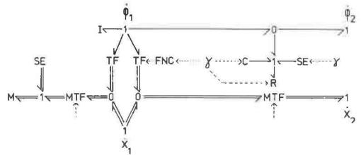
Fig. 2. Bondgraph of a four axial hydraulic knee.
