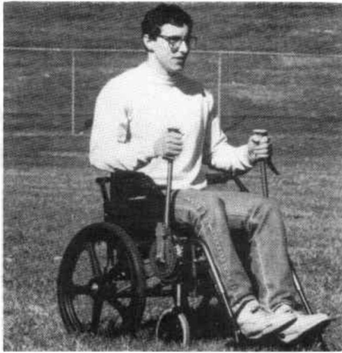
Fig. 1. Experimental lever drive system fitted to a commercial wheelchair. A clutch is operated on each stroke by inward force on the lever, allowing the user to stroke forward, reverse or apply brakes as required.
