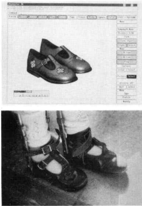
Fig. 3. A Clarks design was mapped over the orthopaedic lasts to produce these custom shoes.
