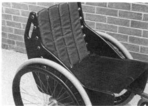
Fig. 10. An experimental wheelchair with the seat, side panels and hand rims produced by NASA. The panels have a foam core with skins of Kevlar and graphite impregnated with epoxy resin.
