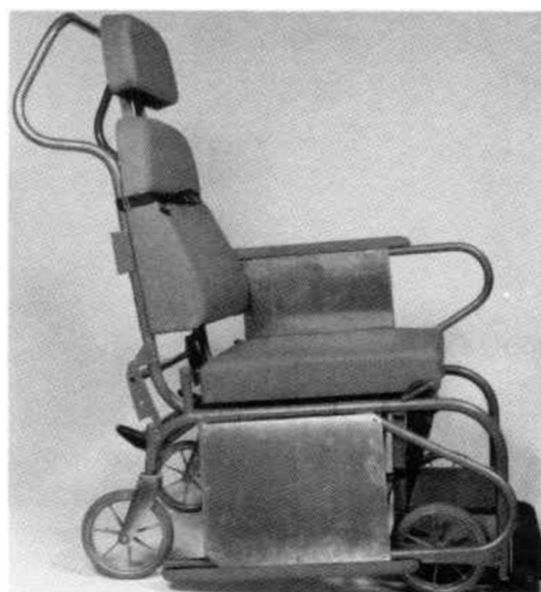
Fig. 6. View of chair showing folded armrests and improved design of pushing handle.
