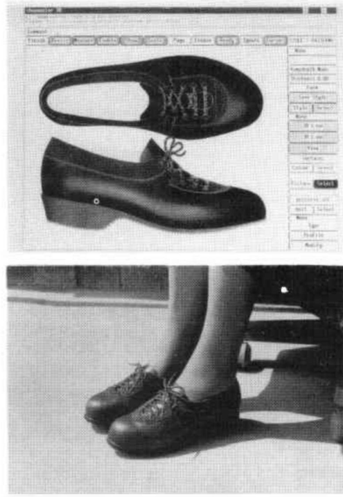
Fig. 4. An example of a screen view and the completed shoe, showing a soft-top feature on a lady's walking shoe.
