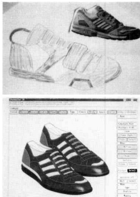
Fig. 2. The design brought in as a free-hand sketch and magazine cut-out, and the corresponding design on the CAD system.
