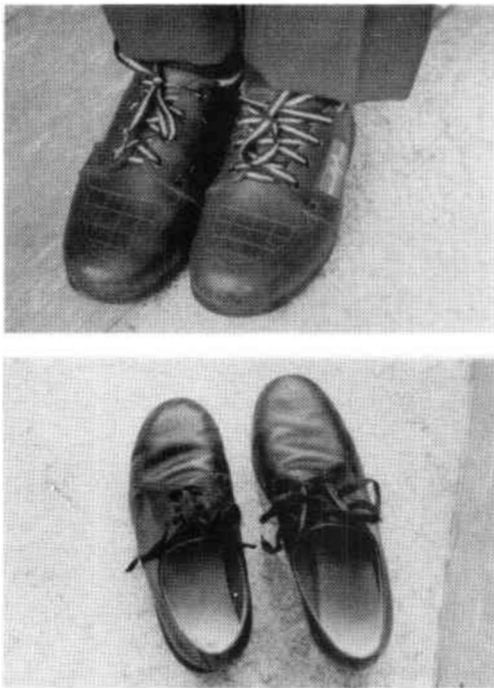
Fig. 5. Comparison of the conventional orthopaedic shoe and trial shoe worn for a similar length of time. The trial shoe has held its shape better, which is thought to be a function of the styling.
