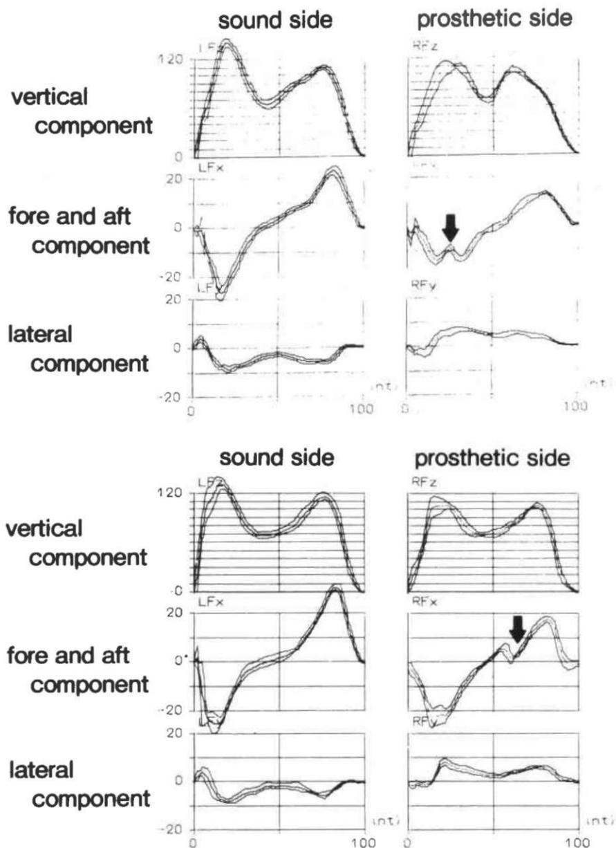
Fig. 1. Irregular wave patterns of the fore and aft component of the floor reaction force. Arrows indicate the irregular wave patterns at the beginning of the heel contact or push-off stage.
