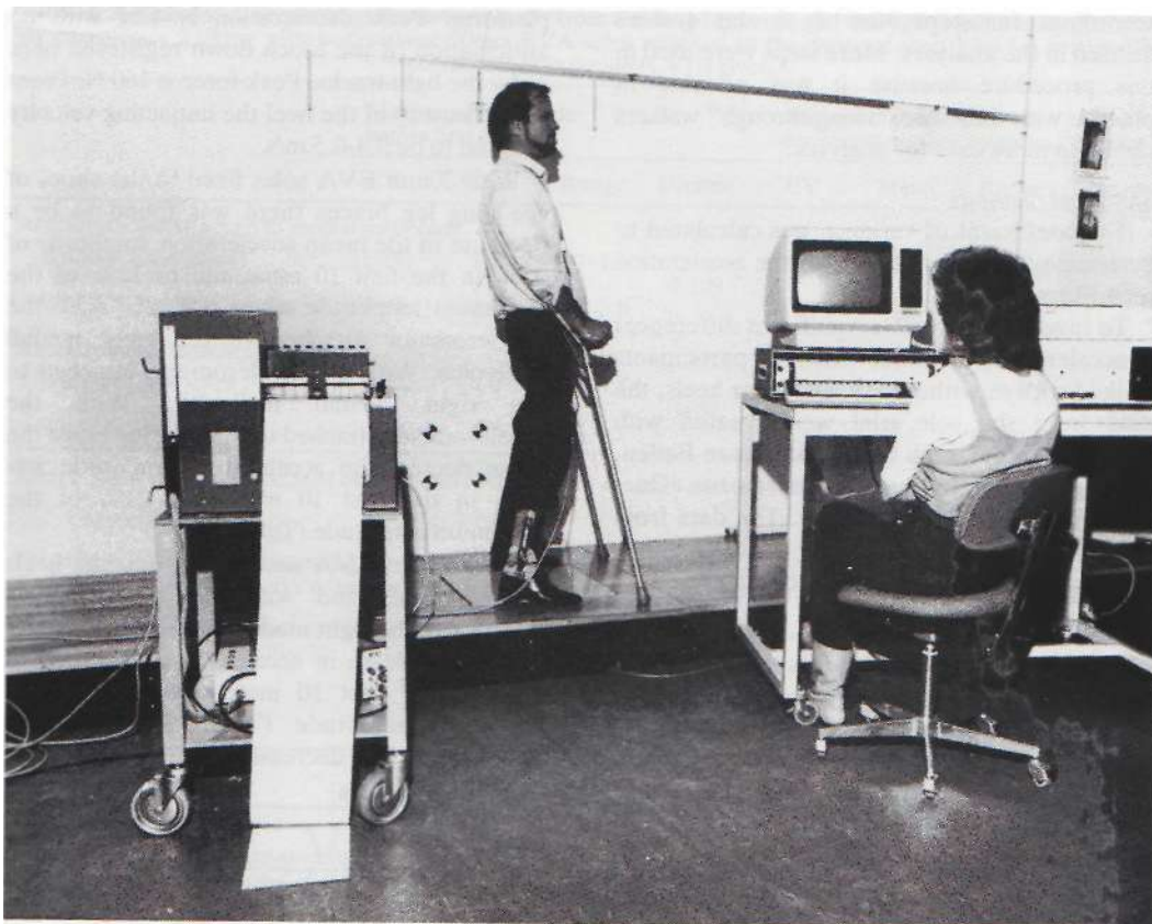
Fig. 2. Paraplegic walking with long leg braces and forearm crutches along a wooden walkway during an experiment with accelerometer attached to the medial malleolus.
