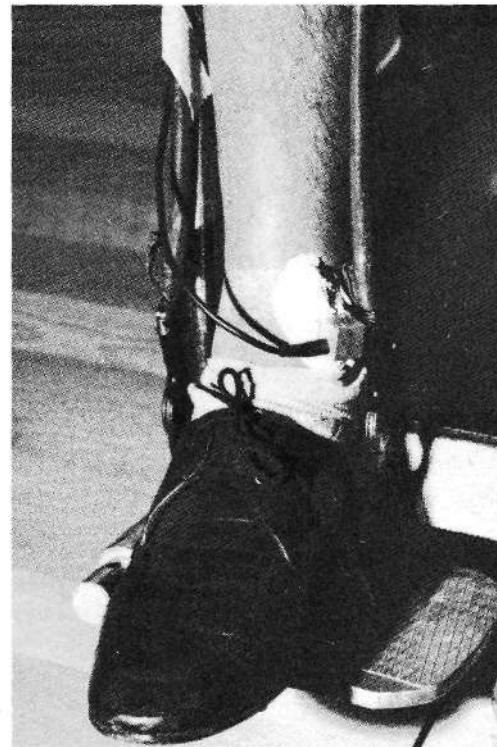
Fig. 1. Accelerometer fixed in a plaster holder and taped to the medial malleolus of the right leg, to create bony contact.
