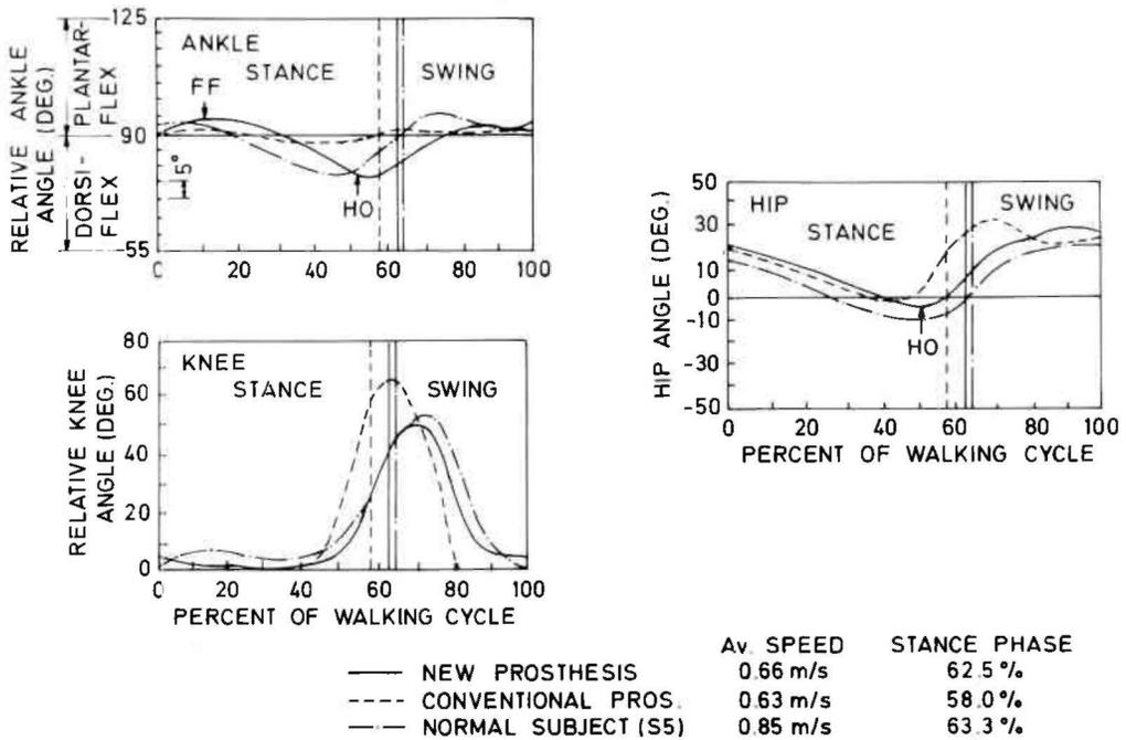
Fig. 10. Relative angular rotations of ankle, knee and hip during amputee walking with (i) new prosthesis and (ii) single knee axis conventional prosthesis and their comparison with the corresponding patterns for normal subjects.
