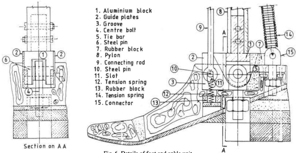
Fig. 6. Details of foot and ankle unit.
