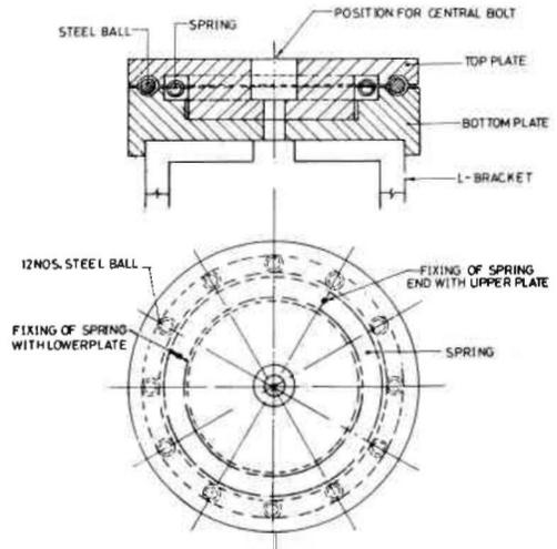
Fig. 5. Details of turntable used for cross-legged sitting.
