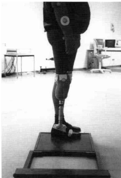
Fig. 1. Measuring the static alignment of a trans-tibial amputee with the "L.A.S.A.R. Posture" system.
