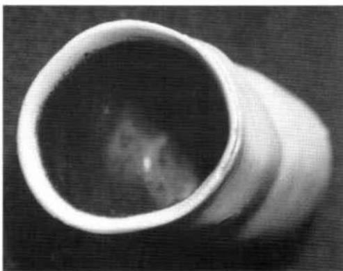
Fig 1. An affected prosthesis showing a black discolouration caused by fungal growth on the internal surfaces.
