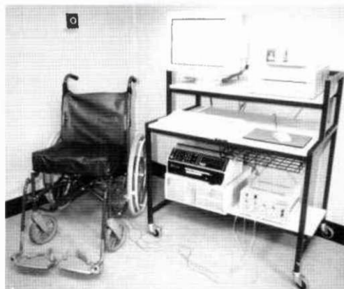
Fig. 1. Equipment used to record air pressure, interface pressure and pressure-time cycle characteristics of the cushions.
