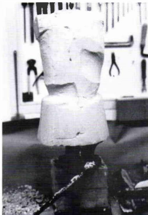
Fig. 1. Plaster positive modelled and corrected.
