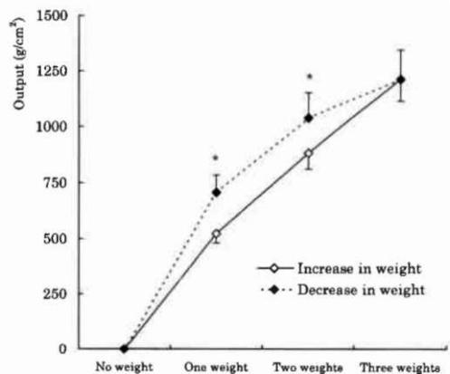
Fig. 3. Hysteresis characteristics of the sensor. Output increased linearly with the loaded weight; however, output was greater when weight was being removed. \*:paired *t*-test, *p*<0.05. No weight: 0.254 kg, one weight: 10.760 kg, two weights: 21.587 kg, and three weights: 32.372 kg.
