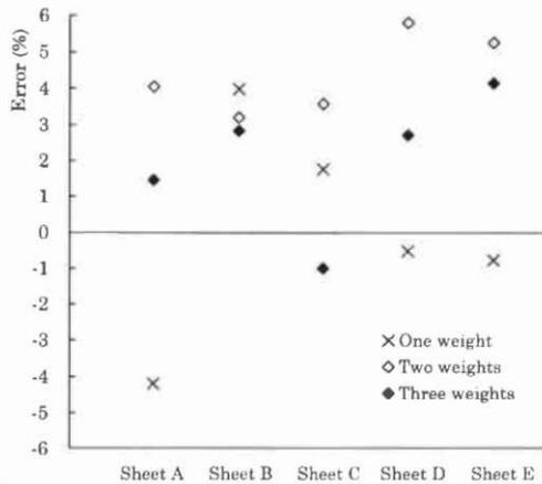
Fig. 4. Error of total output. Error indexes were calculated with the equation  $[\text{output (kg)} - \text{loaded weight (kg)}] / \text{loaded weight (kg)} \times 100$ , and, except two trials, were within 5%. One weight: 10.760 kg, two weights: 21.587 kg, and three weights: 32.372 kg.
