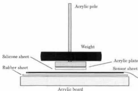
Fig. 1. Lateral view of the apparatus for testing the flexible pressure sensor. The stand for weights is placed on the sensor sheet spread on the rubber sheet covering the acrylic board.
