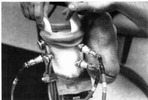
Fig. 1. An instrumented prosthetic socket. Transducers are positioned in mounts at anterior-medial proximal, antero-medial distal, lateral and posterior proximal sites. Dummy transducer plugs fill mounts at sites that are not monitored.
