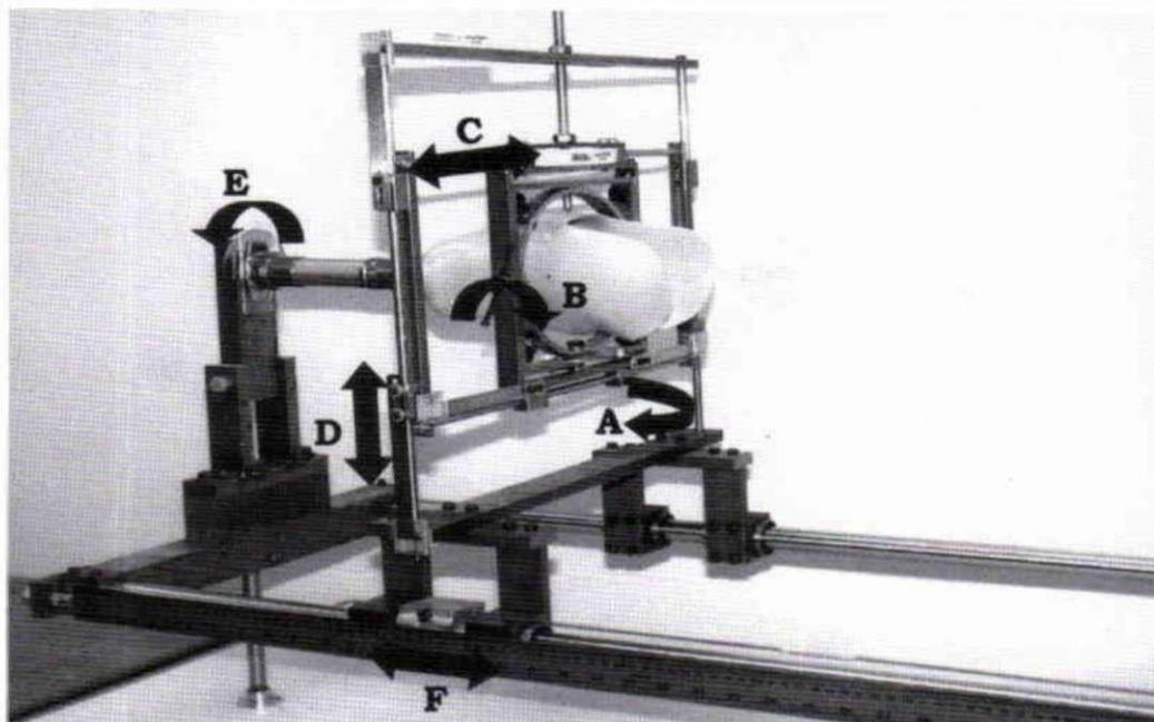
Fig. 2. The mechanisms for inputting the 6 alignment parameters. A – for M/L tilt; B – for A/P tilt; C – for M/L shift; D – for A/P shift; E – for toe-out angle; F – for prosthesis height.
