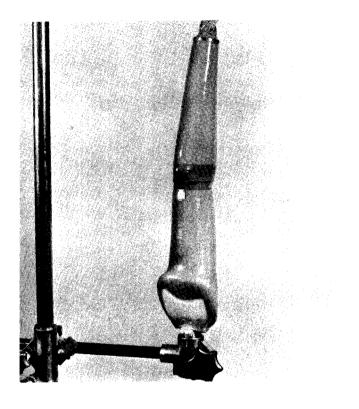
13. Mix polyester resin with its promoter, catalyst and color pigment. (See page). Pour it into the top of the PVA bag and work it into the stockinette. Tie off the top of the bag to remove excess resin. Pull tape around the joint heads to seal off the resin.
