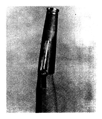
9. Replace the straps and observe the channel made by the material; smooth the edges if needed. The channel under the straps will form space for the layup material. Apply a parting agent on the wax.
