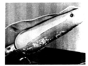
2. After the plaster has set, carefully remove the wax check socket. (Heating the wax with a heat gun will allow easier removal.)
