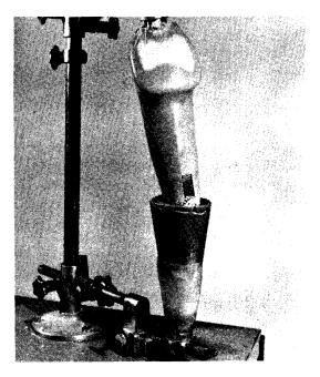
7. Shape the forearm to size by removing the excess material.
