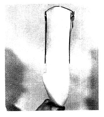
4. Drill the straps for a better bonding of the resin. The distal socket straps can also be soldered together for added strength. Remove the joints and apply the lamination layup. 5. Make and pull over the mold one dacron felt bag. Sew across the ends of 3-inch wide nylon stockinette and pull two layers over the dacron. Tie it at the bottom and cut small holes in the stockinette and dacron to allow the round nuts of the joint spacer to protrude as shown in the illustration
