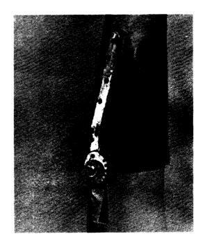
10. Apply two layers of nylon stockinette. Tie the stockinette to the wrist unit groove with string. Cut holes for the joint heads. Fill in with dacron felt any spaces between the straps and the stockinette. It may be easier to remove the joints while applying the first two layers.
