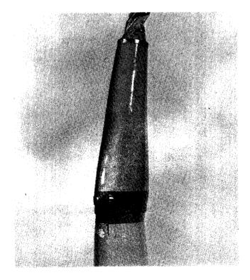
After the resin has set, remove the forearm from the socket and hang the forearm in an oven to melt out the wax. (Temperature of oven depends on kind of wax.)
